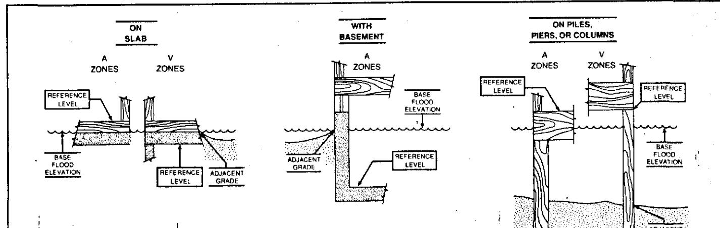
The diagrams above illustrate the points at which the elevations should be measured in A Zones and V Zones.
