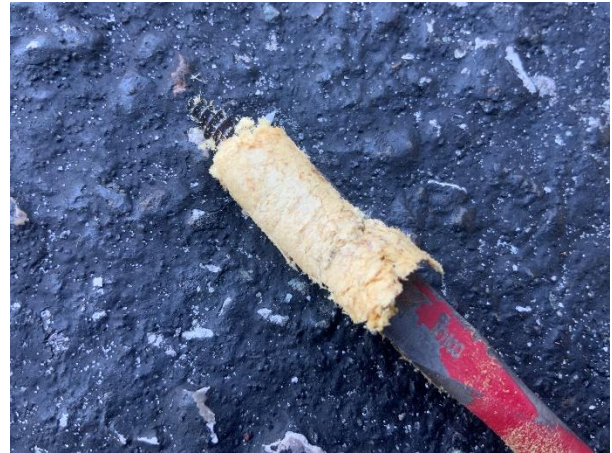
Photo 46 Building 7/8 – West Elevation – Overall view of core sample taken from piling base.
